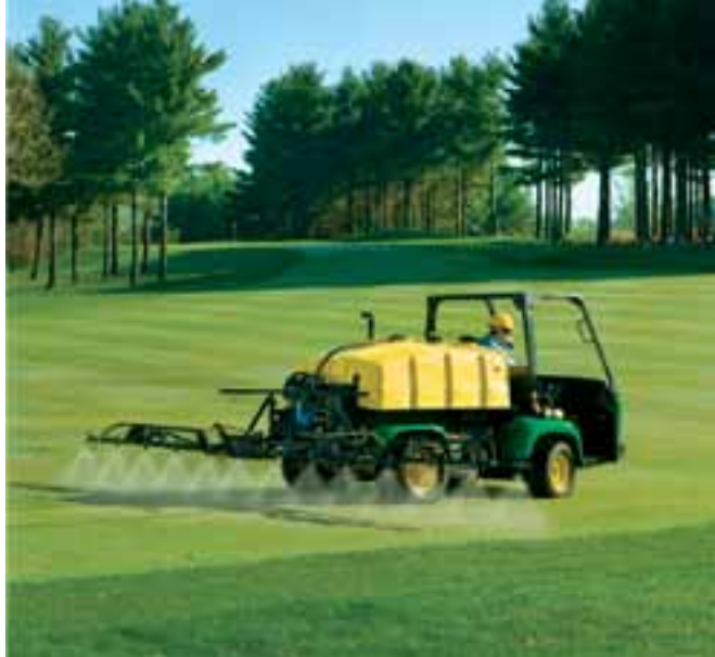
Drift reduction and coverage are two reasons ULD tips are standard on many golf course sprayers.
