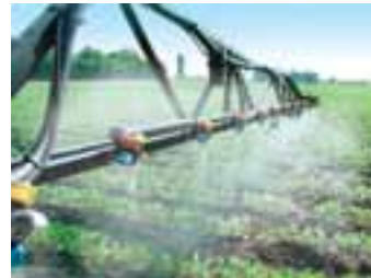
Drift reduction and coverage are two reasons ULD tips are standard on many golf course sprayers.
