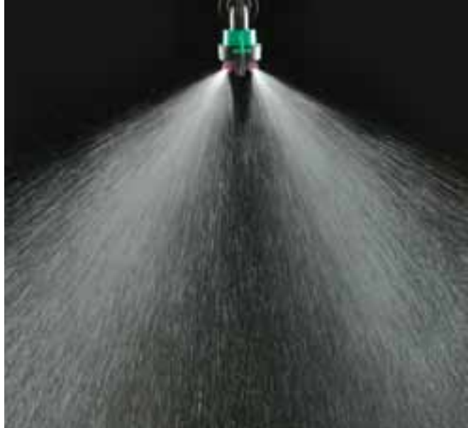
Side view: Two ULD tips placed in a TwinCap tip holder will create a spray zone that is nearly 120 degrees front to back and 120 degrees side to side.
